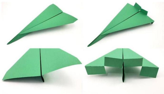
Learners will now change the paper of the paper plane to a thicker paper or add a small object on the top to increase the weight and the force of gravity and decrease the lift. Learners will now measure the distance of flight 3
