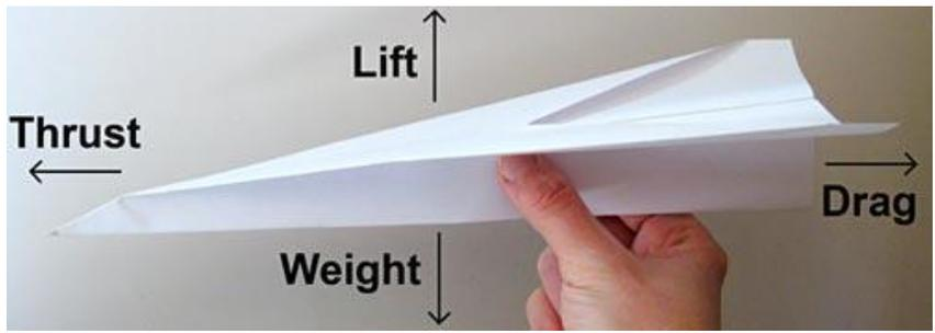
To test thrust: Learners will now throw this plane forward and see it take flight. When you throw a paper plane in the air, you are giving the plane a push to move forward. That push is a type of force called thrust. Thrust can also be achieved by a rotating fan or the flapping wings of a bird. Learners will measure the distance of flight 1
