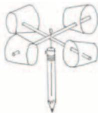
Wind-speed can be recorded based on counting the revolutions (how many times the marked cup comes back to the front) of the anemometer for one minute.
