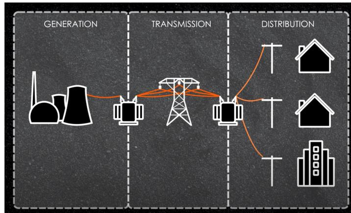
After it is generated, electricity travels through wires into large transformers. The transformers increase **voltage** (the strength of the current), allowing the power to travel far away. The current continues through high-voltage power lines that extend across the area covered by the grid.
